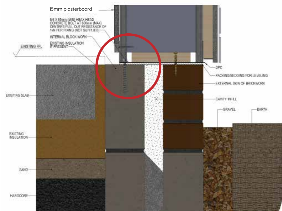
250mm Cavity Wall Base Detail (standard)
