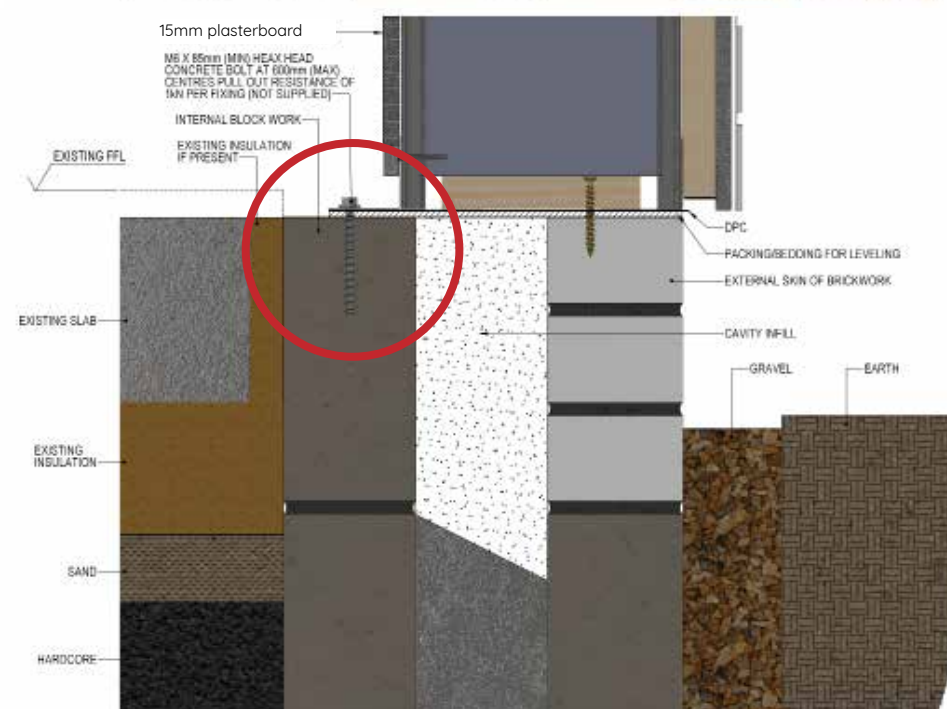
300mm Cavity Wall Base Detail (extended)
